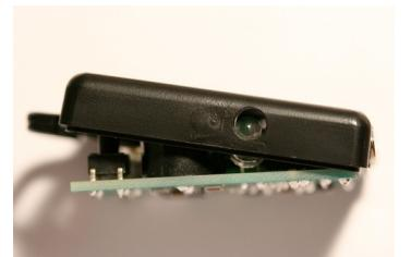
While inserting the PCB the diodes should snap into the side holes and bend to  $90^\circ$ . Use tweezers if necessary.
