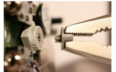
Now, insert the assembled PCB into the enclosure. Remove the **code switch knob** with flat pliers or a knife before. Don't forget to remove the protective seal from the buzzer.
