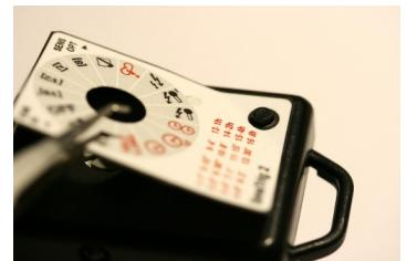
Now the label can be attached. Peel off the protection foil in one corner and align the label (switch, dial) first.
